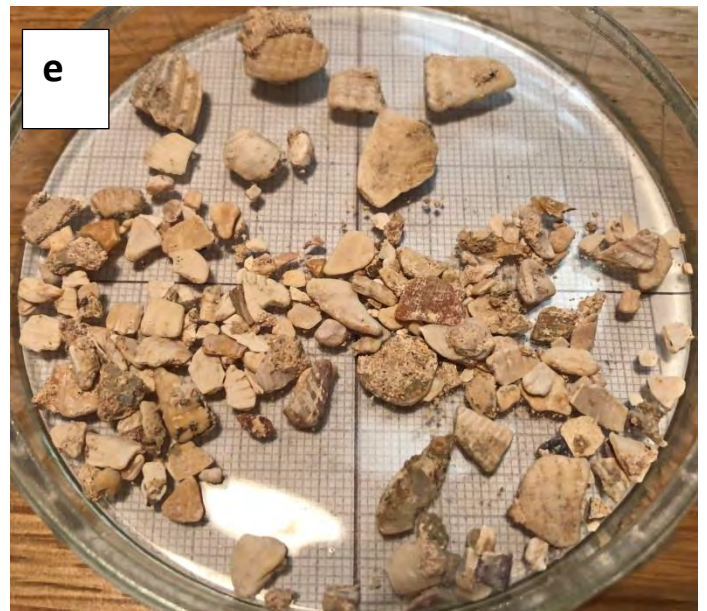
Fig. 6: Lyminge Church mortar Sample 1 (a–c) carbonate replaced plant material; (d–e) marine molluscs; (f) rounded flint beach shingle and gravel. Scales 1mm grid.
