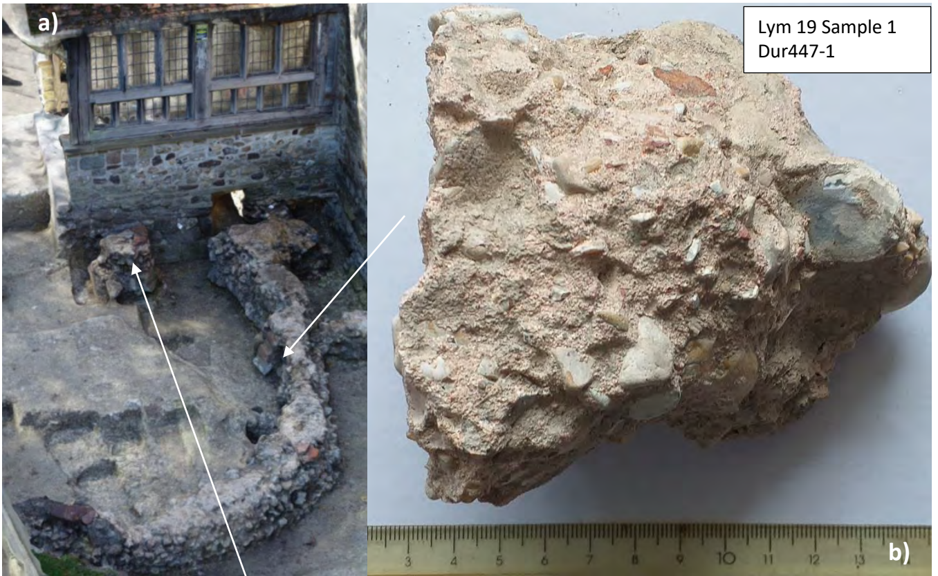
Fig 1a–g. Mortar sample locations and visual appearance
